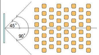
In many events, the width and/or depth of the audience will exceed the ideal viewing area of the image. One obvious solution is to get a larger screen, but often factors such as ceiling height prevent you from increasing the image size. In these situations, placing repeater screens along the parameters of the event space will help the entire audience view the image.
