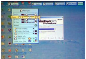
This is a photograph of an image that needs the phase control adjusted. Note the horizontal lines in the background of the image.
