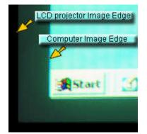
This is a photograph of an image that needs the horizontal and vertical position adjusted.
