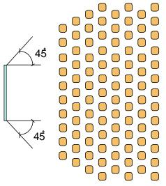
The **good** viewing area is within 45 degrees of the projection axis or within a <u>90 degree viewing cone</u>.
