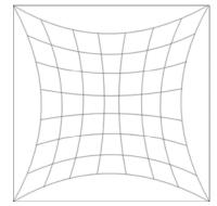
Lens shift may cause a pin cushioning effect, which the image appears to be concave around the edges. Of course, pin cushioning doesn't always appear equal on all sides of the image. If it is combined with a keystone effect, the image may be pin cushioned on only one side. The best solution these optical effects is to properly orient the projector to the screen.
