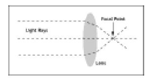
**Fixed Lens** – is a lens with a predetermined fixed focal length without a zoom function. There are long and short throw lenses that are fixed. You must place the projector according to the throw distance specified by the manufacturer, or the image will not focus or fill the screen.
