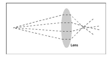
If the projector's image appears to be out of focus in some areas but in focus in others, and you are using the lens shift function, your image may be poor due to spherical aberration. To improve the image put the lens back in the neutral position so that it's lined up with the optics. Move the projector so that it's square to the screen and see if the image improves.
