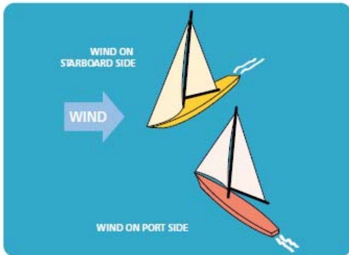
The red sailing vessel gives way to the yellow sailing vessel by either going behind or changing tack to go the other way.
