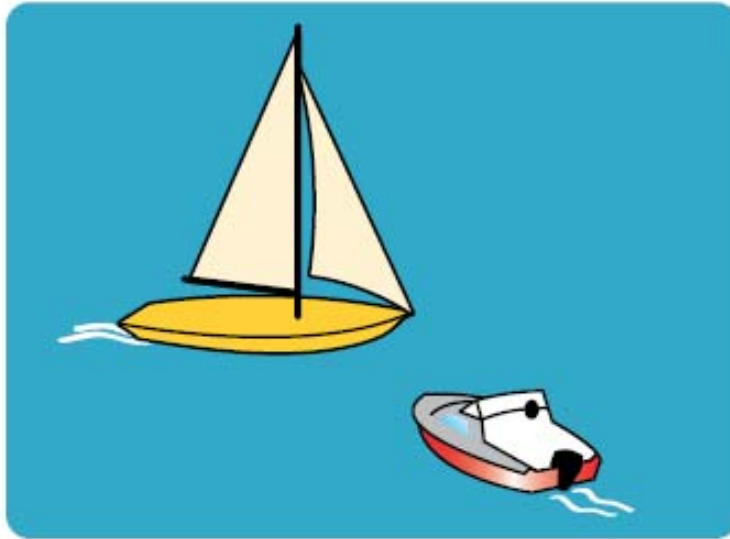
The red powered vessel gives way to the yellow sailing vessel.
