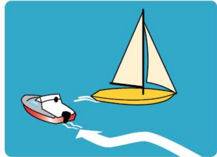
The red powered vessel gives way to the yellow sailing vessel.
